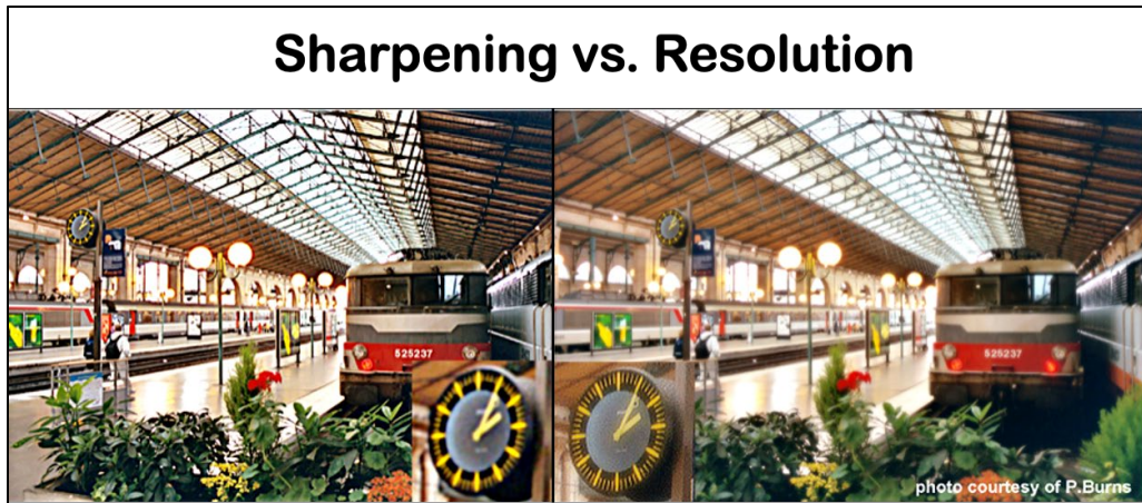
Figure 3: Example difference between sharpening (left) and resolution (right)
