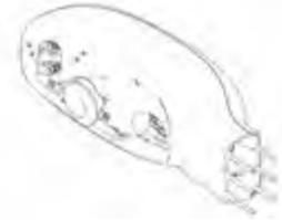
Turn the bulb lock ring counterclockwise and remove the bulb. Do not allow the glass of the new headlamp bulb to come into contact with anything. The glass could become contaminated and cause bulb failure. Reassemble in reverse order.
