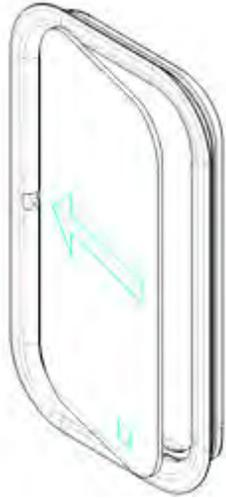
When the forward edge of the glass reaches the forward inside edge of the seal, the glass should pivot outboard into the remaining seal (see arrow in next illustration).
