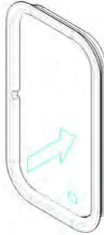
Press and slide the glass into the aft portion of the seal to seat it.
