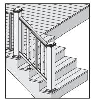
» POST TO POST SPAN WILL BE LESS THAN 6' OR 8'. PRIOR TO INSTALLING POSTS CALCULATE POST TO POST SPAN USING A MAXIMUM RAIL LENGTH REQUIRED AND THE ANGLE (32°-37°) AT WHICH THE RAILS WILL BE INSTALLED. DO NOT INSTALL STAIR POSTS AT 6' OR 8' SPAN, AS STAIR RAILINGS WILL THEN BE TOO SHORT.
