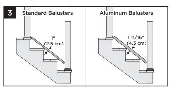
3. If using standard balusters, place a 1" (254 mm) deckboard on the nose of the stair tread. If using aluminum balusters, use a scrap piece of wood measuring at least 1-11/16" thick, and place on the nose of the stair tread.
