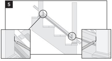
5. Use the lower and upper stair post to set the length of the bottom stair rail. Ensure that baluster spacer holes are spaced evenly between posts. Also allow for a minimum of 1-1/2" (292 mm) at each end of the stair rail for bracket placement and baluster clearance. Mark rail at post intersections.
