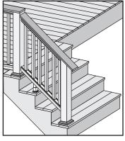
» DO NOT CUT POST/POST SLEEVES UNTIL TOP RAIL IS FULLY INSTALLED. THE DECK BOARD USED IN TRANSCEND STAIR COCKTAIL RAILING WILL NEED TO TERMINATE AT THE TOP OF THE POST AS SHOWN ABOVE. THE DECK BOARD WILL HAVE TO BE INSTALLED INTO THE SIDE OF THE POST IN THESE AREAS USING 2 APPROPRIATE COMPOSITE DECKING SCREWS - PRE-DRILLING IS RECOMMENDED.
