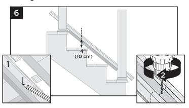
6. Mark approximate location for foot block, allowing a measurement of 4" maximum. Invert the bottom rail, and at marked location drill a hole using a 3/16" drill bit in the center of the channel. Foot block is to be installed at last step. For spans over 6' in commercial applications, mark and drill two locations spaced evenly apart for two foot blocks.
