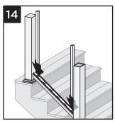
If using rail gaskets, subtract 1/16" from each end and cut. KEEP BALUSTER SPACER IN
