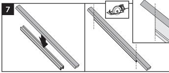
7. Using the cut top rail as template, cut 2x4 at same angle and length of the top rail.
