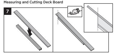
7. Using the cut top rail as template, cut deck board at upper post location at same angle as the top rail. Leave a generous amount of deck board material at lower post location as this will allow for overhang and can be cut later.
