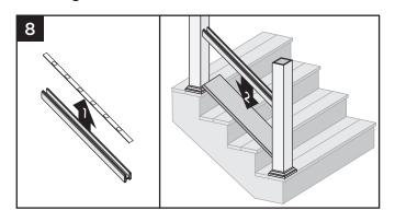
8. Remove baluster spacer from bottom rail and place rail in between posts, keeping rail on deckboard.
