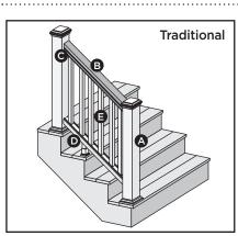
Cutting post sleeves is **NOT** required. Ensure both top and bottom post/post sleeves are tall enough to accommodate top rail and 2" x 4" (51 mm x 102 mm).
