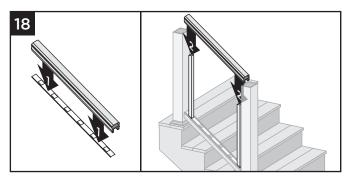
18. Remove baluster spacer from top stair rail and place rail in between posts on top of balusters, ENSURING that balusters remain parallel to post.
