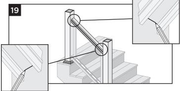
19. Mark both posts on inside channel of the top stair rail. Remove top stair rail.
