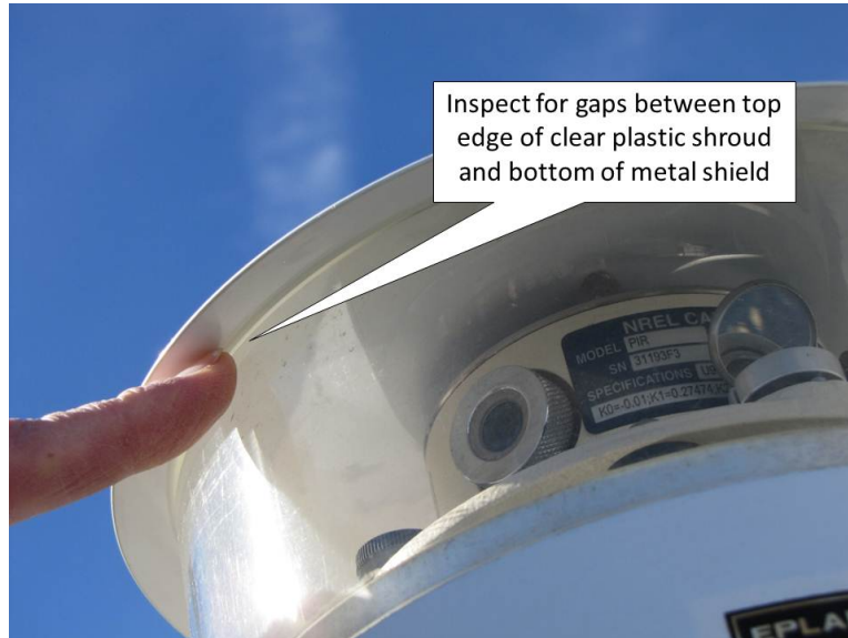
Figure 24. Inspecting for gaps under the sun shield.
