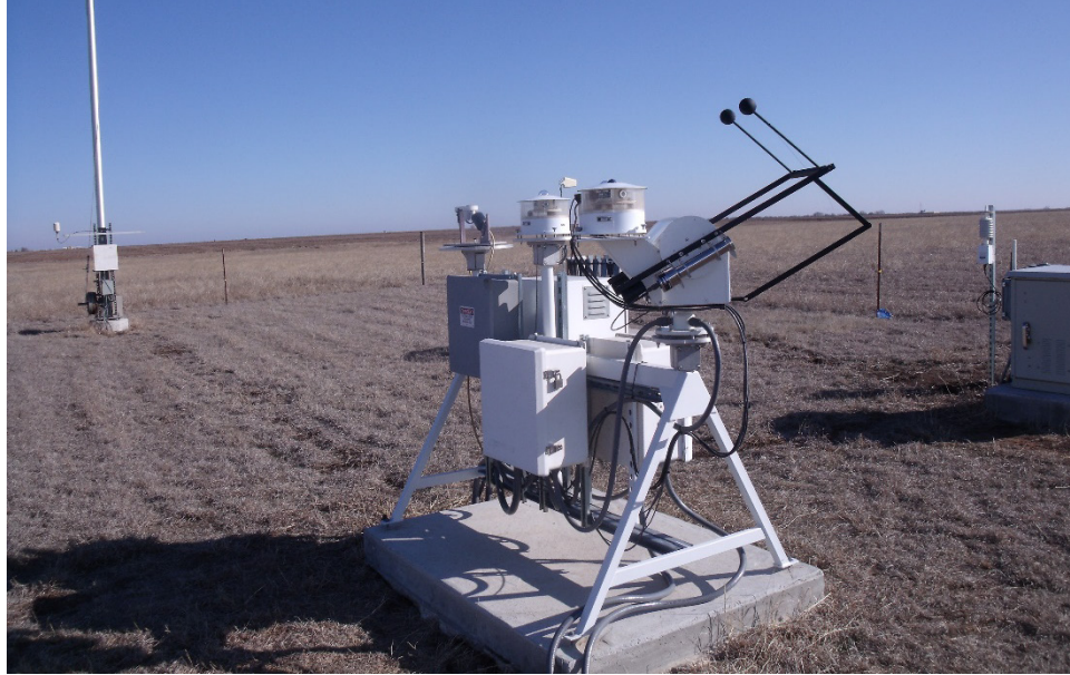
Figure 1. SIRS radiometers for downwelling irradiance measurements.
