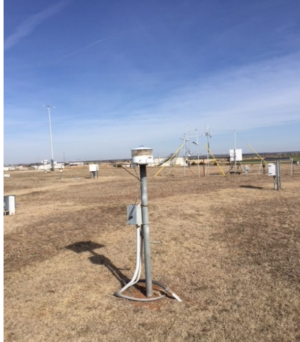
Figure 5. Single global PSP radiometer on pedestal at the SGP BRS site.
