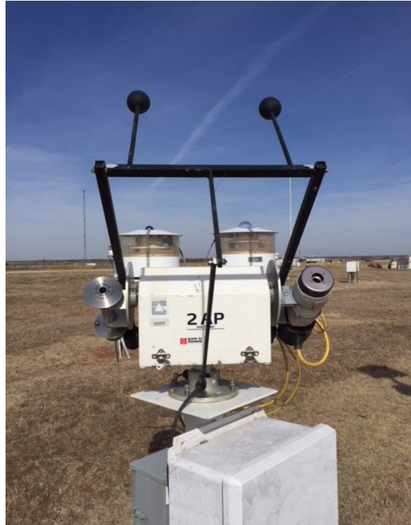
Figure 4. Tracker-mounted PIR, 8-48, and NIP radiometers at the SGP BRS site.
