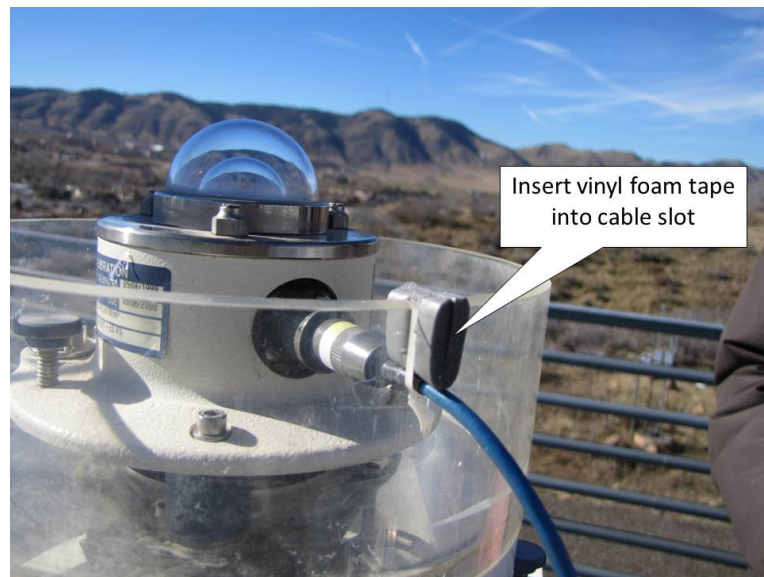
Figure 23. Plugging the slot with foam.
