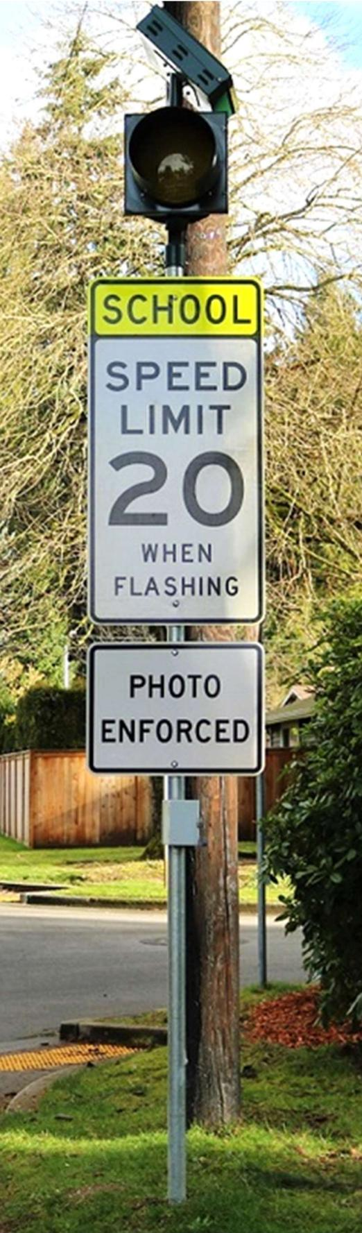
**Signage:** The purpose of SSC is to encourage safe speeds, and the law requires that signs notifying drivers of speed safety cameras be installed at least 30 days prior to activation of the camera. The signs must inform drivers that they are entering an area where speed violations are enforced by an automated traffic safety camera and must follow the specifications of the Manual of Uniform Traffic Control Devices.
