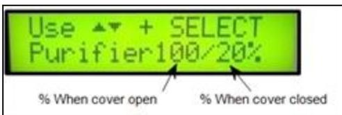
**Example with the Retractable Pool Cover Open and the Temperature Display on.**
