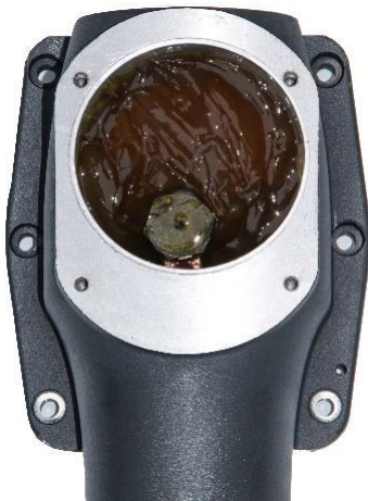
Figure 4: New grease example (before any single use)
