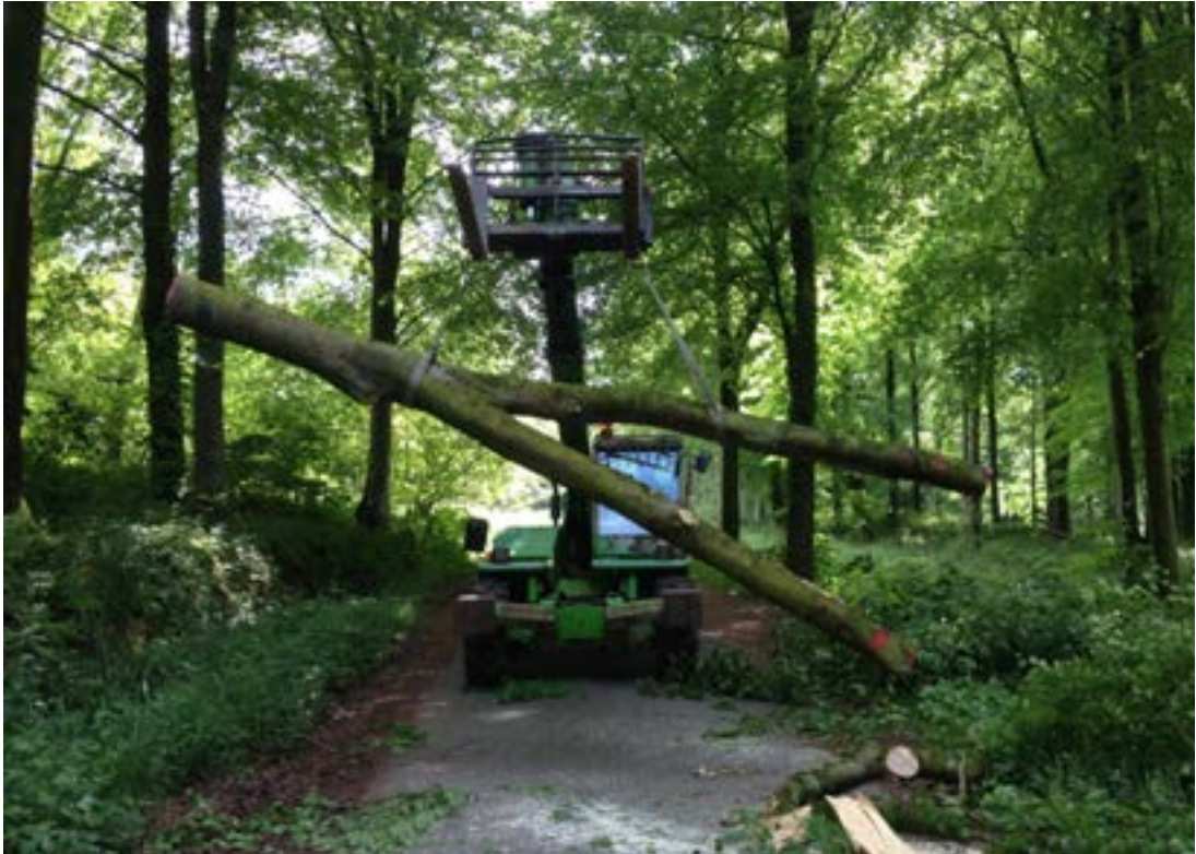
Fig. 11. Fork 12_A03. Cut to a length of five meters in the woods, forks wanted to be kept as large as possible to ensure flexible use, while also kept manageable - weighing approximately 500kg at this length
