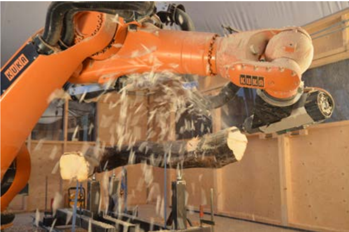
Fig. 18. The robotic arm machining a bearing surface on to a forkB stem. While limited to a milling head for the scope of this project, future endeavours will likely use multiple tool heads.
