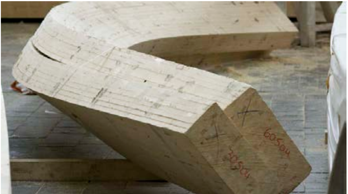
Fig.4, 5. The Metz Pompidou is a spectacular contemporary wood structure. Yet each component is made by first reducing trees to squares sections of approximately two cm before having a complex form returned to it.
