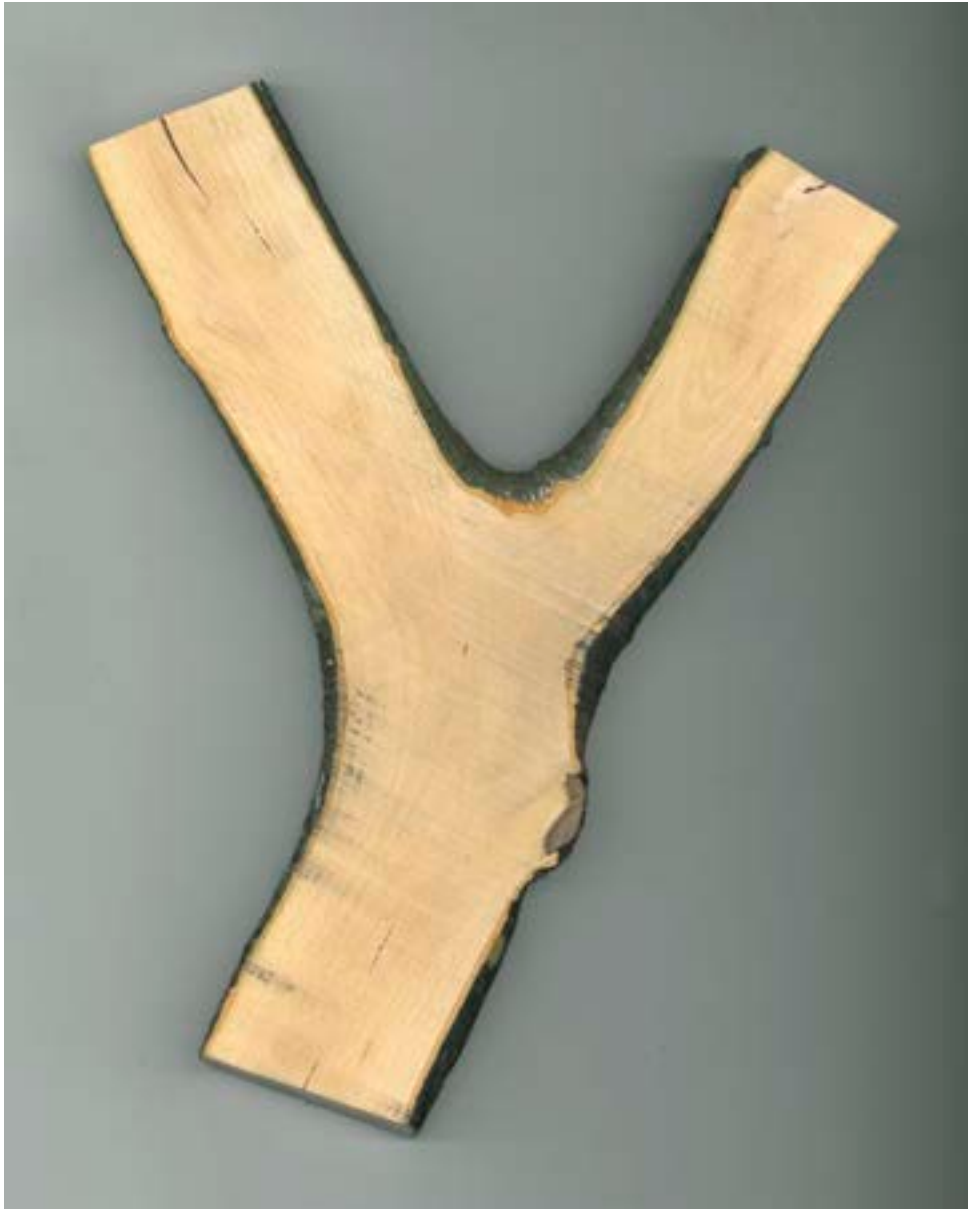
Fig. 8. Placed on a scanner after being sawn in half, this image gives some sense of multi-directional grain structure present within forks.
