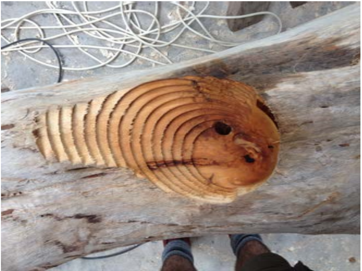
Fig. 19. The mortise and tenon connection designed for the Tree Fork Truss. While involving basic mechanical fasteners, this joint implies the potential to revisit complex wood to wood jointing with digital tools
